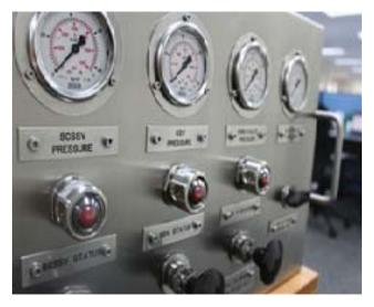
**The Well Control Panel** is a pneumatic/hydraulic control unit designed to safely operate for sample the three main safety valves (SSSV, SSV & SCSSV installed on a producing well. Not limited to this, it is also used to operate other actuators and valves. The unit can be sized in accordance to customer's requirements to control the number of wellheads.
